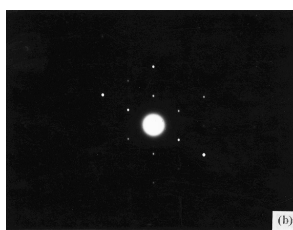
Figure 3 Morphology of one pauci chain single crystal of gutta percha (a) and its corresponding electron diffraction pattern (b)
