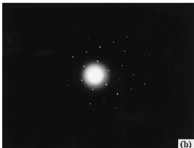
Figure 1 Morphology of one single chain single crystal of gutta percha (a) and its corresponding electron diffraction pattern (b)
